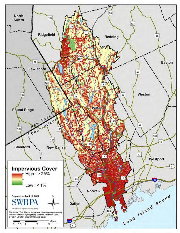
Figure 3-4. Watershed Impervious Cover
