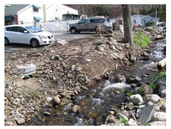
Near-stream development can mean that runoff from parking areas is piped directly into the stream
