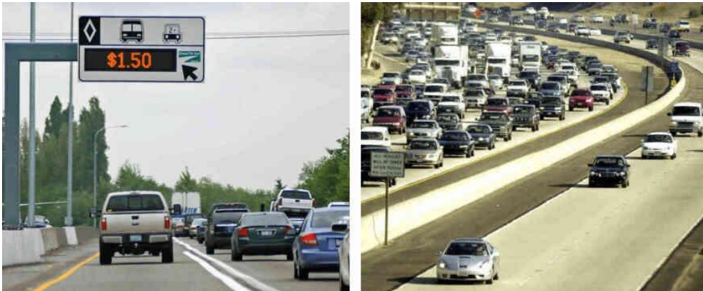
Photo at left shows electronic toll amount as driver approaches the HOT lane access zone. The toll on the sign increases as traffic gets heavier. Photo at right shows pleasant driving conditions in the HOT lane - for those who can afford it.
