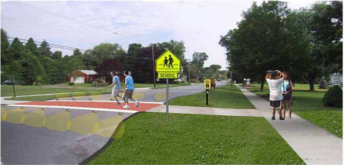
Proposed Enhancements: Raised-textured crosswalk, in-pavement lighting, curb-extensions, improved school zone signage, and reconfiguration of the Middle School main driveway.
