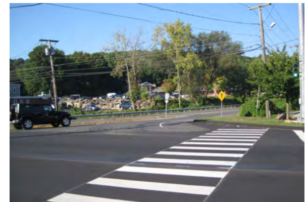
Crosswalk at Route 7 and 102 Pedestrian crossings at Route 7 are limited, in this example the crossing lacks curb ramps and does not have a dedicated pedestrian phase or pedestrian signal heads.
