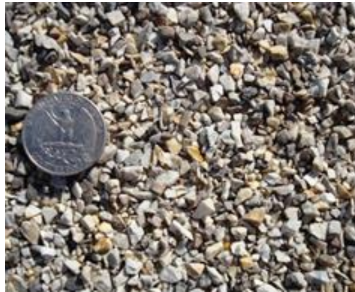
Figure 17. High Friction Surface Treatment (Source: FHWA)
