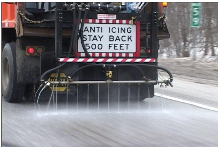
Figure 7: City of Sheboygan Wisconsin Anti-Icing Operations with Stream Type Nozzles
