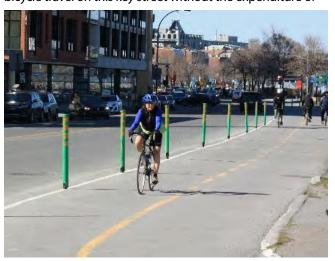
Figure 1 - Low-cost bike lane in Montreal using flexible lane delineators. Photo credit: Dave Sousa.
