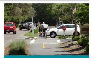
Trails are substantially different from sidepaths. Sidepaths are aligned along a roadway, typically within the roadway rightof-way, and often require users to frequently cross intersections, decreasing safety.
