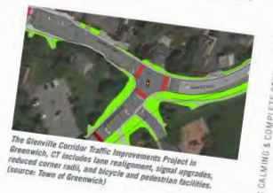
The Glenville Corridor Traffic Improvements Project in Greenwich, CT includes lane realignment, signal upgrades, reduced corner radii, and bicycle and pedestrian facilities. (source: Town of Greenwich)
