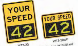
MUTCD standards for speed feedback signs (W13-20 and W13-20aP; source: MUTCD)
