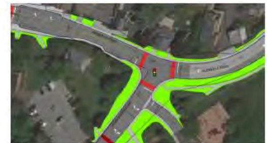
The Glenville Corridor Traffic Improvements Project in Greenwich, CT includes lane realignment, signal upgrades, reduced corner radii, and bicycle and pedestrian facilities. (source: Town of Greenwich)
