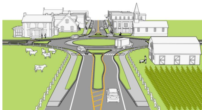
Figure 3 Transition from Rural to Main Street with a Roundabout Gateway (Source: Toole Design)
