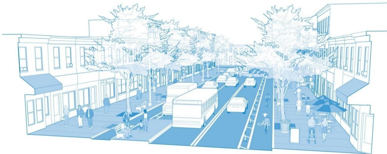
Figure 6 Example of a Complete Street, featuring facilities and amenities for people walking, biking, rolling, driving, or taking transit, as well as freight vehicles (Source: Toole Design)
