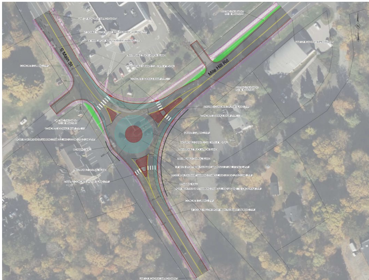
Figure 2. S. Main Street at Mile Hill Road Project Concept Design of Proposed Project (complete concept package included in Appendix D: Project Concept Designs)
