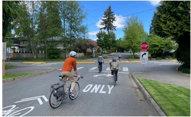
Forced turn island with through-access for bicyclists in Kirland, WA
