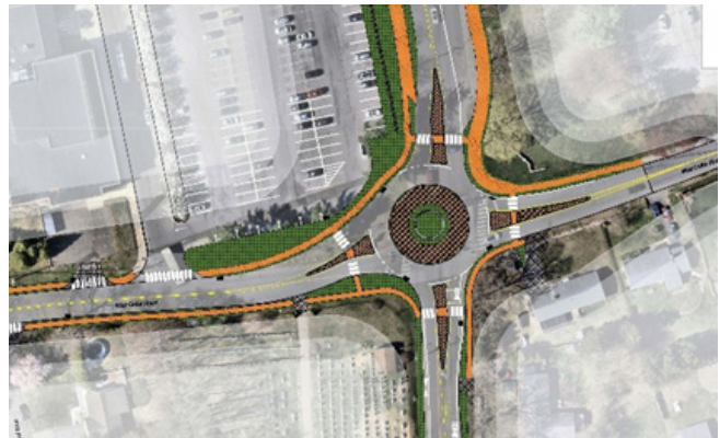
Roundabout Concept for Richards Avenue at W. Cedar Street in Norwalk, CT (source: UCONN - CTI)
