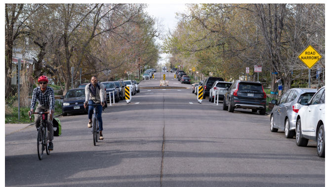
Lane narrowing on a residential street in Denver, CO
