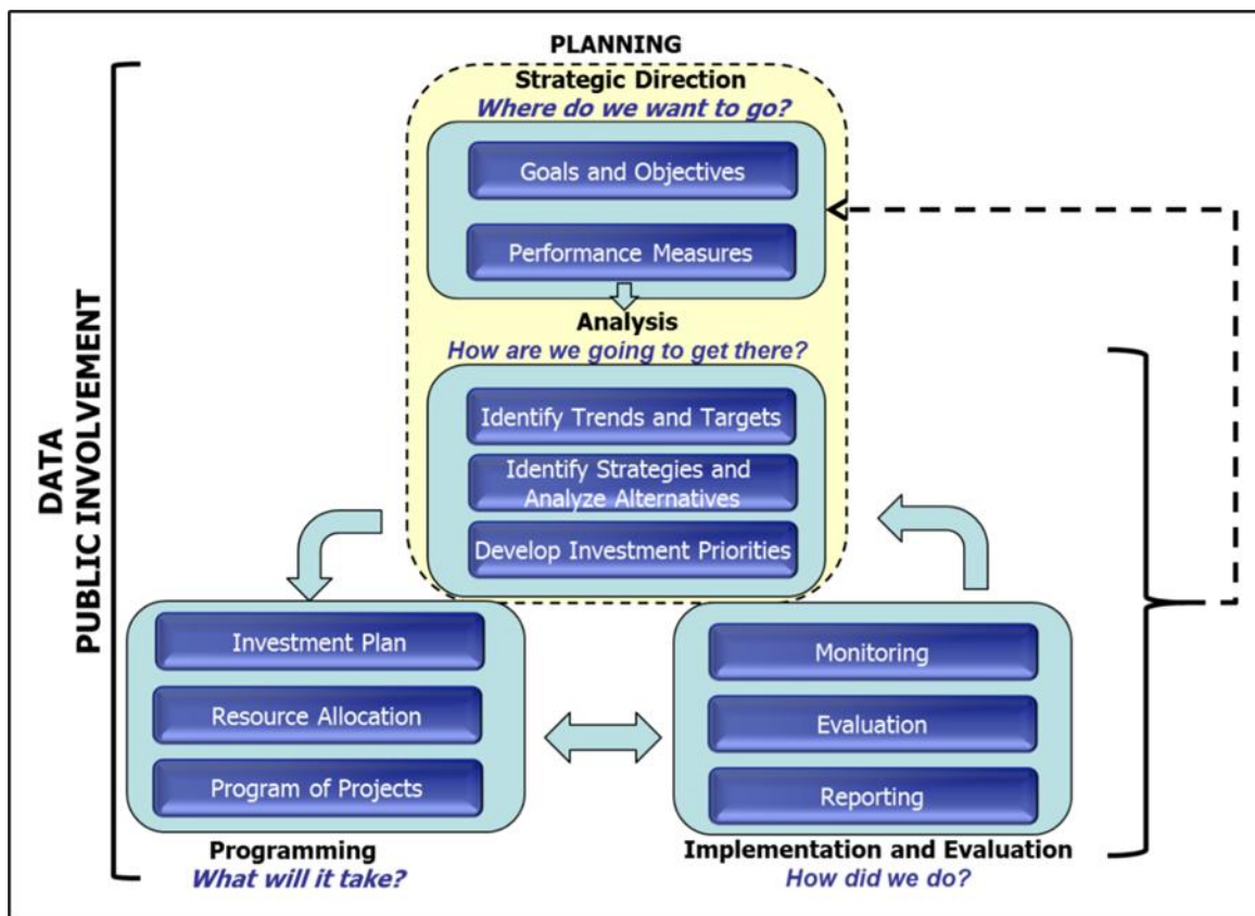
Figure 11. Performance-Based Planning Process (Source: FHWA, Performance-Based Planning and Programming Guidebook, page 14)
